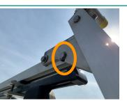
The 'Roller Head' is the triangular end section of your system
